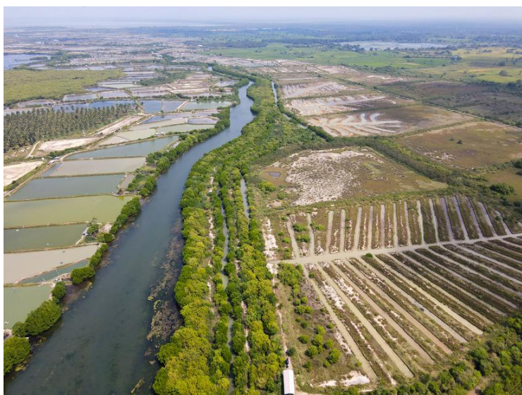
Figure 1. Newly excavated straight and contoured channels to restore hydrology and condition the soil. Active shrimp farms are in the other side of the sanctuary. (© WNPS)
