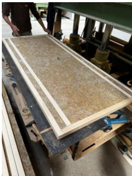
Figure 2. a) Prototype inner door panel made from paludiculture biomass. (© Baufritz)
