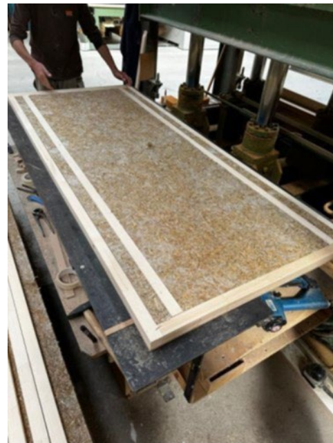
Prototype inner door panel made from paludiculture biomass. (© Baufriz)
